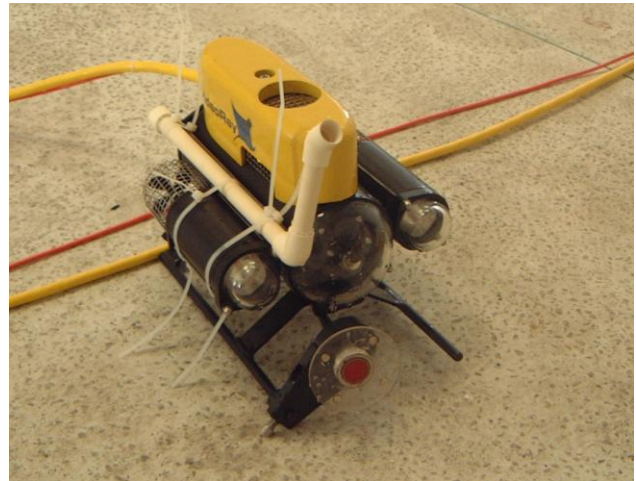
Figure 6. Micro-OCROV with Ultra-sonic Metal Thickness Gauge Attached
