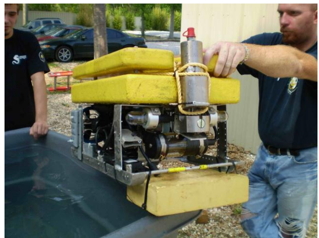
Figure 10. OCROV with Hydraulic Wire Cutter
