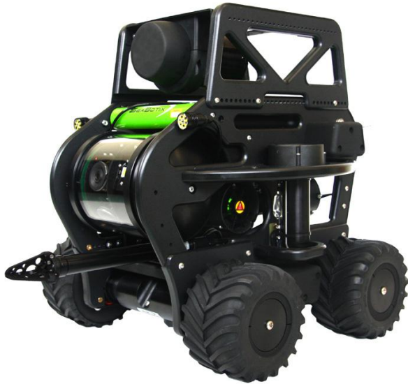
Figure 12. LBV150SE-5 Bottom Crawler Configuration
