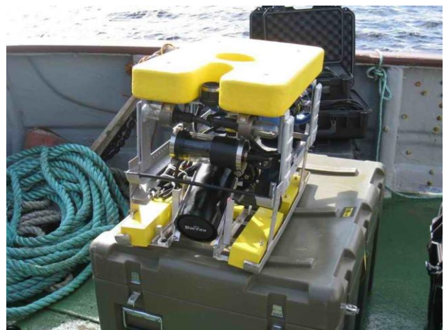
Figure 11. OCROV with Multibeam Sonar
