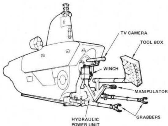
Fig. 9 The WSP as it would appear mounted to the Alvin manned submersible
