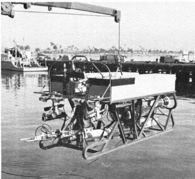
**Fig. 3** The CURV III with ordnance recovery claw installed
