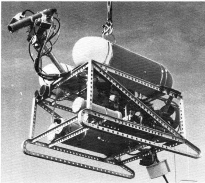
**Fig. 2** The SCAT being launched prior to underwater television inspections
