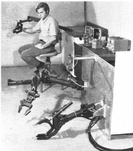
Fig. 7 The RUWS manipulator suit during laboratory testing
