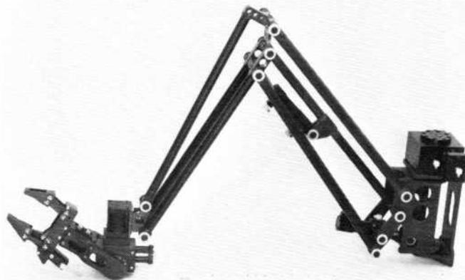
Fig. 11 The seven-function "linkage" manipulator
