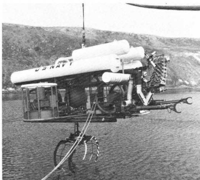
**Fig. 12** Work System Package/Pontoon Implacement Vehicle
