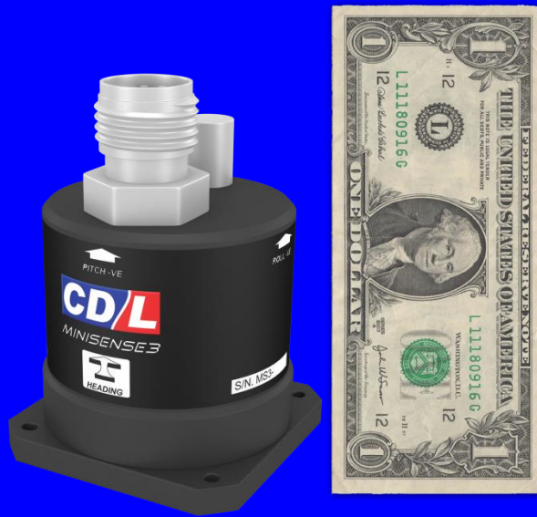
The CDL MiniSense 3, a 2 degree magnetic Aided Altitude and Heading Reference System – Courtesy CDL
