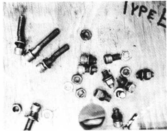
Figure 5. Effect of a 2" drop of the WSP on 11 of its 16 mounting bolts.
